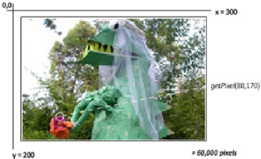
Figure 9. An illustration of the way in which a bitmap graphic is represented numerically and its pixels can be accessed individually with the getPixel() method
